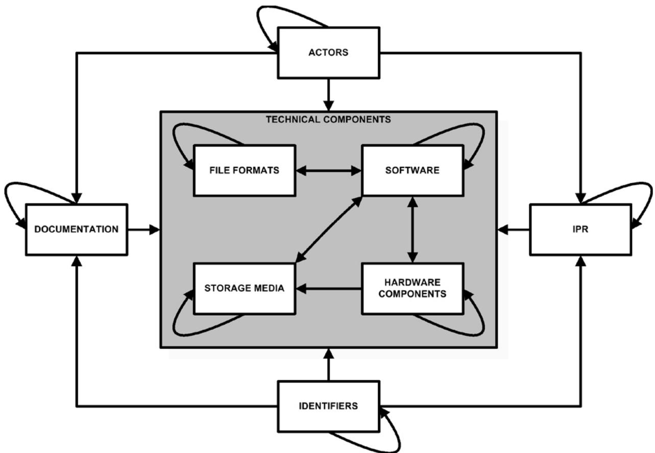
At the heart of the model are the various types of inter-related technical components which are required to model the technical environment of a digital object. Associated entities describe the actors, documentation, intellectual property rights, and identifiers which relate to these technical components and each other.
